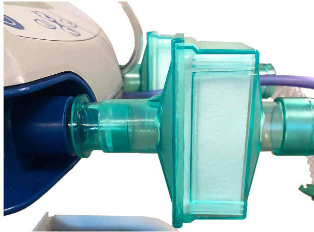
Figure 4-11. Close-up of Exhalation Bacteria Filter Connection
