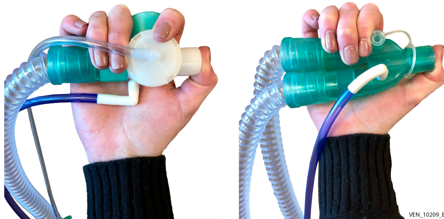
Figure F-4. Blocking the Patient Circuit (single-limb circuit at left; double-limb circuit at right)
