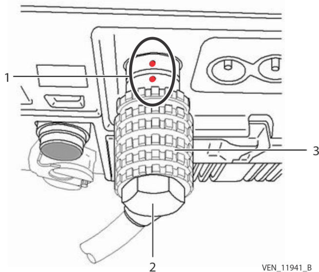
Figure 6-5. Connecting the DC Power Cable to the Ventilator
