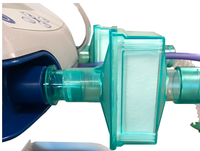
Figure 6-11. Close-up of Exhalation Bacteria Filter Connection
