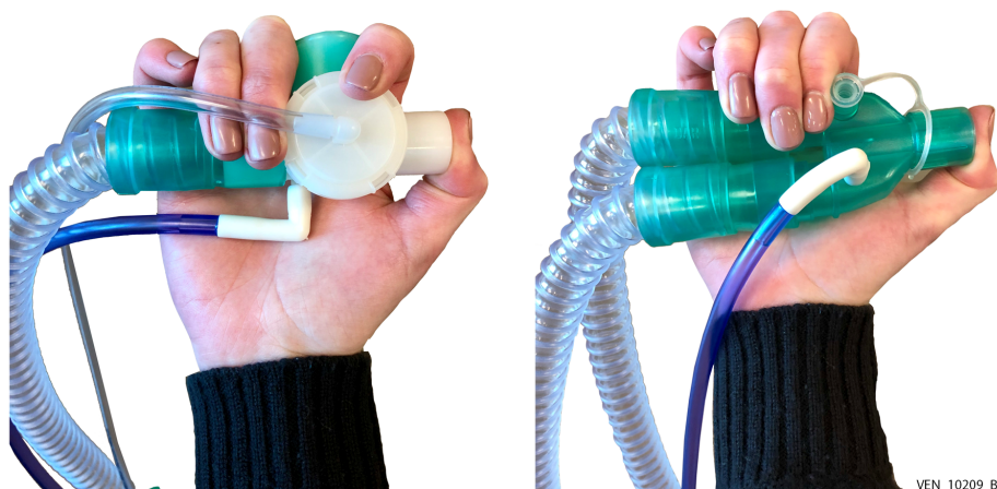
Figure F-10. Blocking the Patient Circuit (single-limb circuit at left; double-limb circuit at right)
